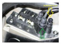
(3) Take care about wiring in this step. A mistake can cause serious damage to the MSO or to the bike. Connect red marked MSO cable instead of the blinding plug. Connect other two MSO cables between the speed sensor to and the motor unit using corresponding connectors.
