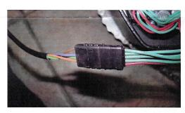
③ Connect both appropriate connectors from the MSO instead of the original connectors into the the motor unit and, firmly press the original, previously disconnected connectors into the MSO according to the color coding (red wire side onto the red/orange wire side, or down-facing at the motor body).
