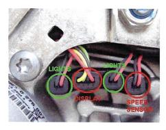
appropriate Connect both connectors from the MSO instead of the original connectors into the the motor unit and, the original, previously disconnected connectors into the MSO according to the color coding (red wire side onto the red wire side).
