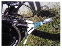
④ Place the MSO in a proper position (we reccomend into the e-bike frame, if possible) and optionally, fasten the wiring using the electrical ties. Fold back the motor and fasten the previously removed INBUS screws. Reattach the plastic cover and the bike is ready to go.
