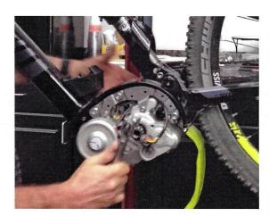
② Disconnect the 4-position connector in between the display unit and motor unit (marked as DISPLAY on the picture) aswell as the 2-position connector in between the tacho sensor and motor unit (marked as SPEED SENSOR).
