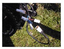
3 Connect all four appropriate connectors on the MSO into the four, previously disconnected, mating connectors on the e-bike. All the conectors have a keying which prevents wrong connection, there is only one way all of them can be connected.
