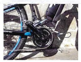
(2) Disconnect the 4-position connector in between the display unit and motor unit and the 3-position connector in between the tacho sensor and the motor unit.
